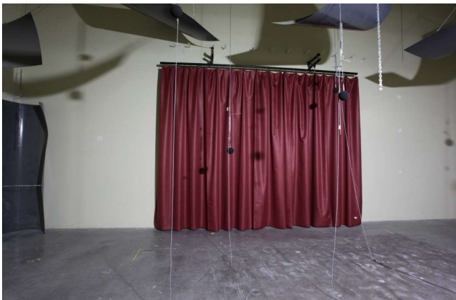
Distance d = 150\text{mm} (G150-mounting) Height [H] = 3050\text{ mm} Width covered surface = 4000 mm Pleated curtain : 180%, total width of the fabric = 7200mm
