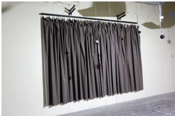
Photo Test 1 : Curtain SOFTLINE_G100_300% pleated_floc at the front
